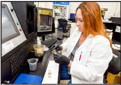
**CORPUS CHRISTI ARMY DEPOT, Tx.** – Oil analysis is crucial for maintaining readiness and ensuring flight safety in Army aviation. Regular laboratory testing of used oil samples assesses the lubricant's condition and serves as an early warning system to predict equipment breakdowns. At the heart of this essential process is the Corpus Christi Army Depot, home to the Army's only aviation depot oil laboratory.
